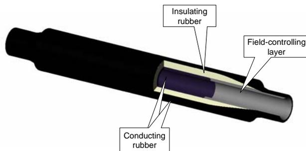
Figure 6. Prefabricated DC joint
