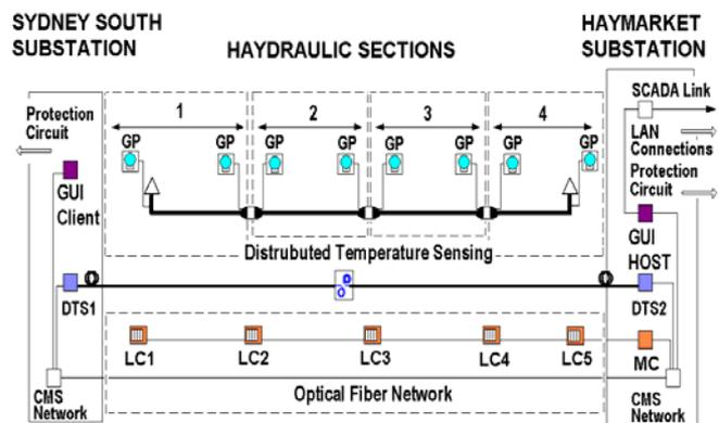
**Fig. 8. Diagrammatic Representation of CMS Functions**
