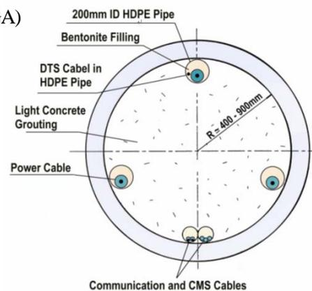
**Fig. 9. Cable Installation in Micro-tunnel**
