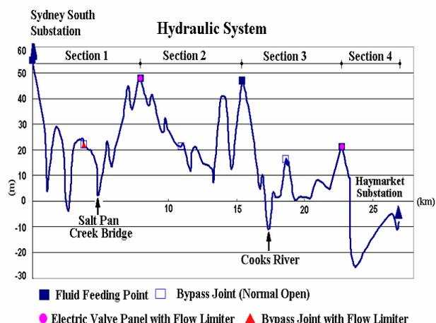
**Fig. 2. Hydraulic Profile of Cable Route**
