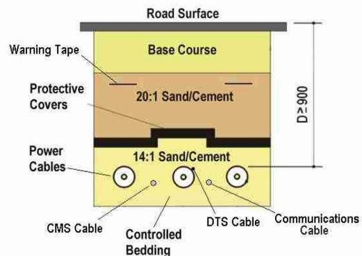
**Fig. 4. Installation of Cable Circuit in Flat Formation**
