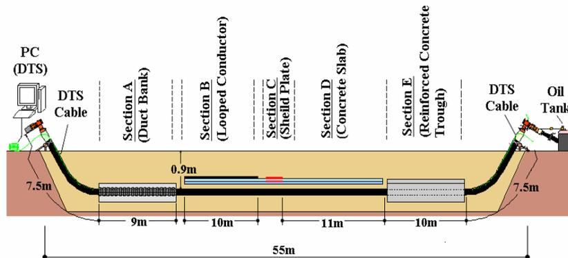
**Fig 7. EMF and Temperature Profile Test Layout**
