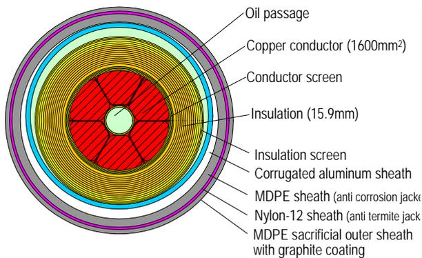
**Fig. 3. 330 kV PPLP Cable**
