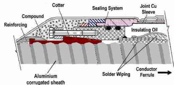
**Fig. 5. Internal Wiping System**
